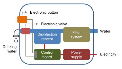
The water disinfection reactor can be seamlessly integrated into your system with the help of a faucet and other accessories, including a flow switch and control board. This comprehensive solution offers a convenient and user-friendly interface, making it an excellent choice for a wide variety of applications.
